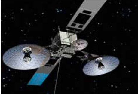
Satellites like this Tracking and Data Relay Satellite (TDRS) have large antennae and solar panels that deploy once they are in orbit. © Boeing. All Rights Reserved.
